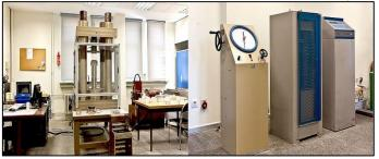
In this laboratory physical and mechanical properties of rock samples, taken from the surrounding rocks of underground structures (galleries, tunnels, underground openings) and natural building stones like marble, travertine, are determined.
