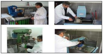
This laboratory is used to prepare rock specimens for mine machinery and mechanization laboratory in order to determine the cuttability and wearability of rocks.
